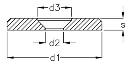
$\begin{array}{ll} \text{Countersunk screw} = \text{M4} \\ \text{d1} & = 20 \\ \text{d2} & = 4.3 \\ \text{d3} & = 8 \\ \text{s} & = 3.0 \\ \end{array}$
